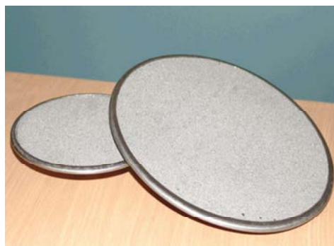
Fig. 2: The aerator of sintered titanium powders [3, p.120]
